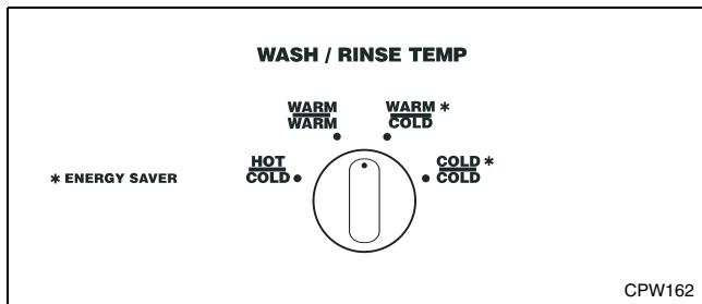
There are four WASH/RINSE temperatures available – HOT Wash/COLD Rinse, WARM Wash/COLD Rinse, WARM Wash/WARM Rinse, and COLD Wash/COLD Rinse.
